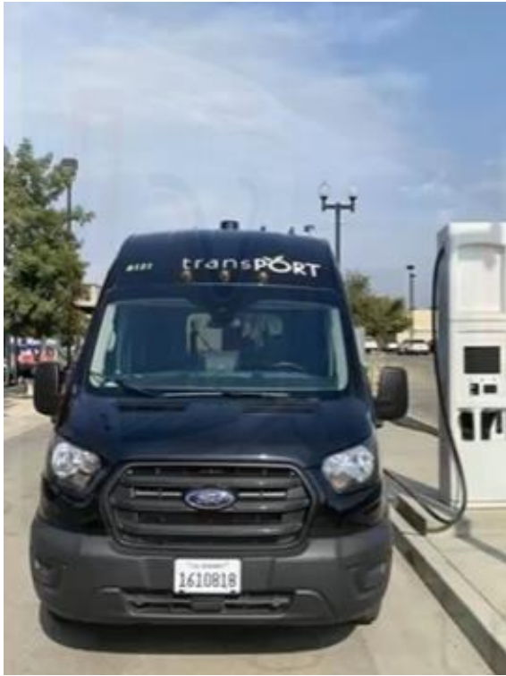
Figure 20: A BEB Passenger Van Plugged into a Charger.
