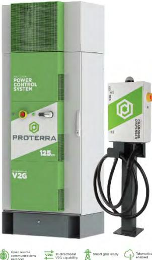
The CalACT/MBTA Vehicle Purchasing Cooperative offers two version of the Proterra Energy Charging System that operate on 480V. Both charging systems are capable of charging a single standard ZEB vehicle battery in approximately three hours and can support up to four additional charging dispensers to charge additional vehicles simultaneously, however, charging multiple vehicles at the same time increases overall charging time. Proterra charger
